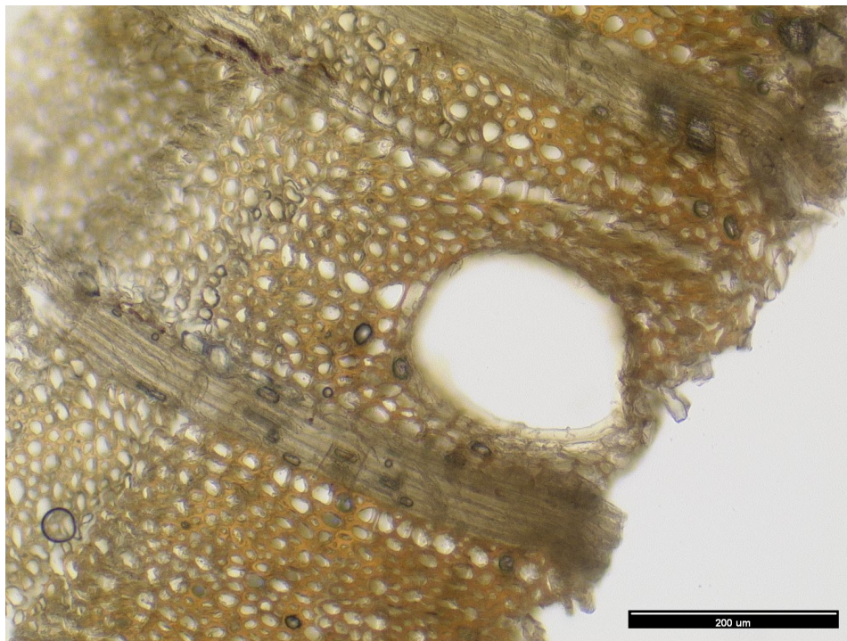
Figure 2. Axial section showing vessel representative of the diffuse porous structure. Typical vessel width is greater than half of space between rays, yet wider than the rays.
